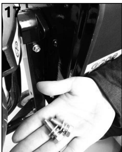
Step 15: Install 2 screws M8*60 and nuts in the circled holes.
