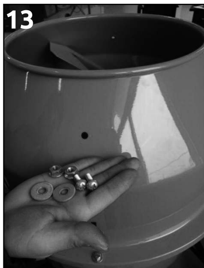
Step 13: Install 2 sets of screw M8*16 & washer M8 outside and 2 nuts inside to fix the top of the mixer blades.
