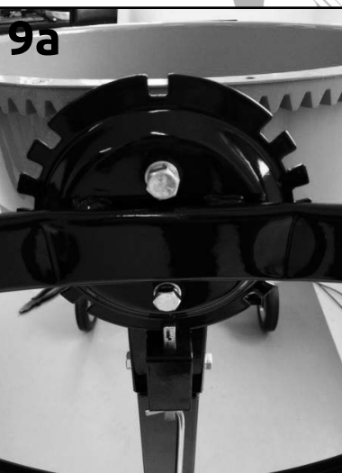
Step 9: Assemble the steering wheel. Use 2 sets of screw M8*16 & spring washer M8 & washer M8 as shown to fix.
