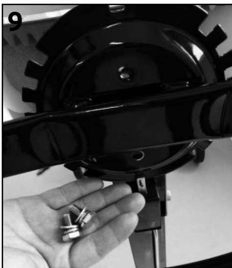
Step 8: Install the tie rod, washer M6, spring washer M5 and 2 nuts M5 in order as shown, tighten the 2 nuts M5 to fix the tie rod.
