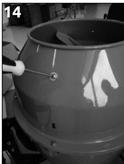
Step 14: Tighten the screws and nuts with tools as shown.
