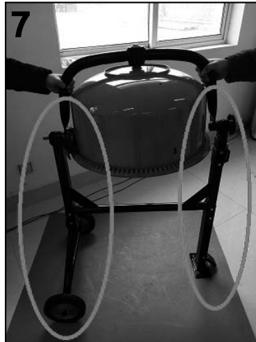
Step 7: Two people take out the lower drum by holding the 2 sides of the curved bracket and put in place as circled.
