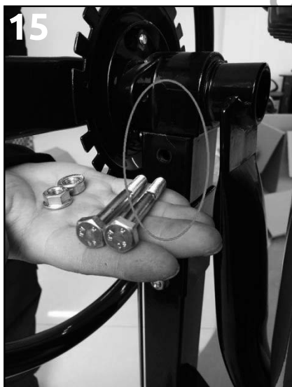
Step 15: Install 2 screws M8*60 and nuts in the circled holes.
