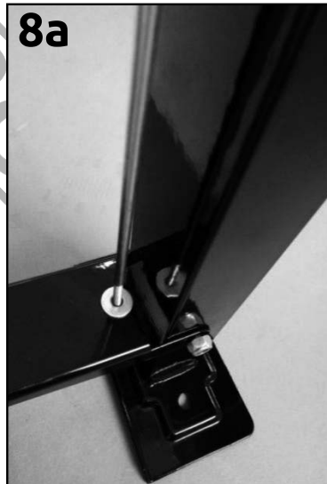
Step 8: Install the tie rod, washer M6, spring washer M5 and 2 nuts M5 in order as shown, tighten the 2 nuts M5 to fix the tie rod.
