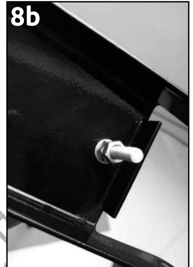
Step 8: Install the tie rod, washer M6, spring washer M5 and 2 nuts M5 in order as shown, tighten the 2 nuts M5 to fix the tie rod.
